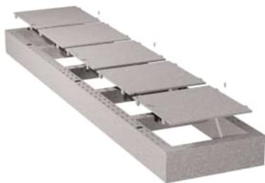
Beams Coffers Install Detail
