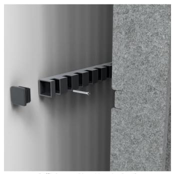
Baffle Systems Direct Mounting Detail
